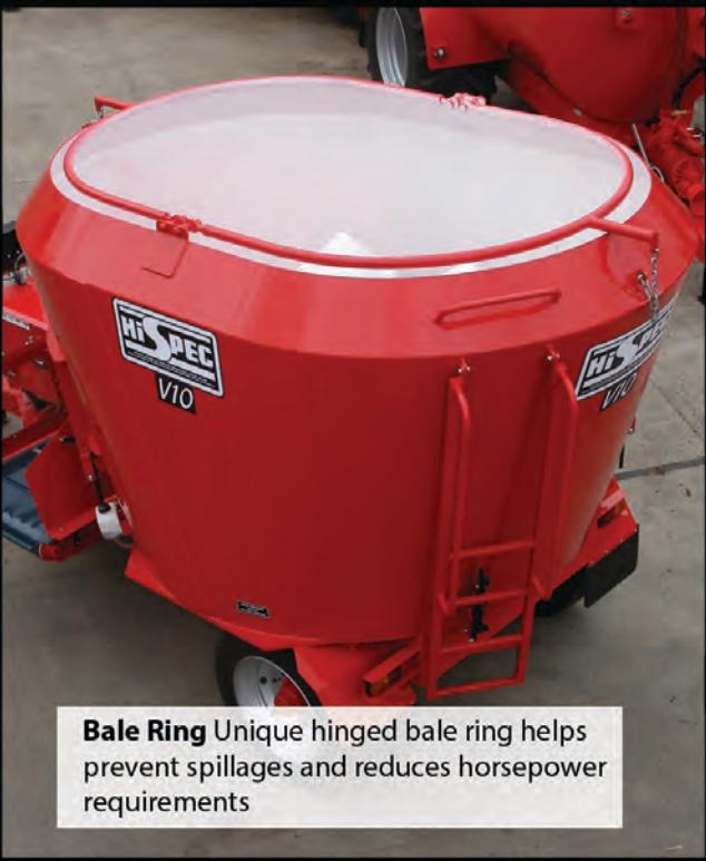
**Bale Ring** Unique hinged bale ring helps prevent spillages and reduces horsepower requirements
